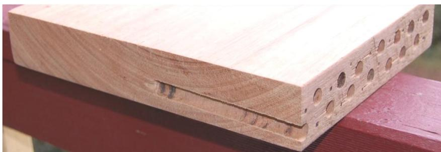
Figure 3. Burrows drilled across the wood grain.
