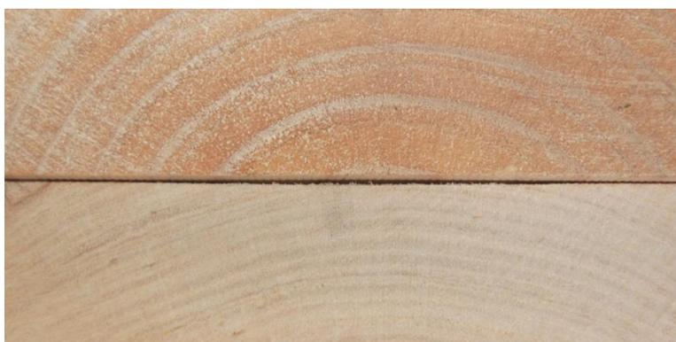
Figure 2. Soft wood (top) compared to hardwood (bottom).
