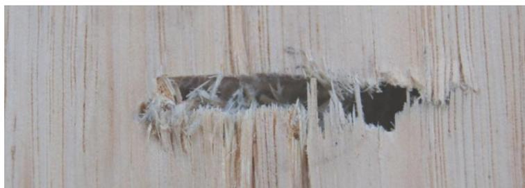
Figure 8. Side of block ripped open by crooked drill bit.
