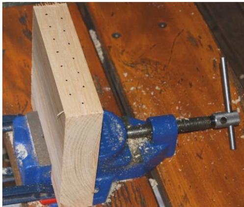
Figure 6. Marked wood block secured in vice.
